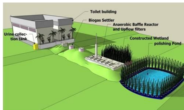
Fig.1 the diagram shows the construction of the biogas plant in a very clean way. It consists of - waste (urine, and other) collector tank, settler of the biogas, anaerobic reactor, and the constructed wetland.
